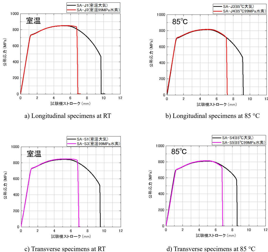
Fig. C.1.9.3 Stress - stroke curves of SA-723.
