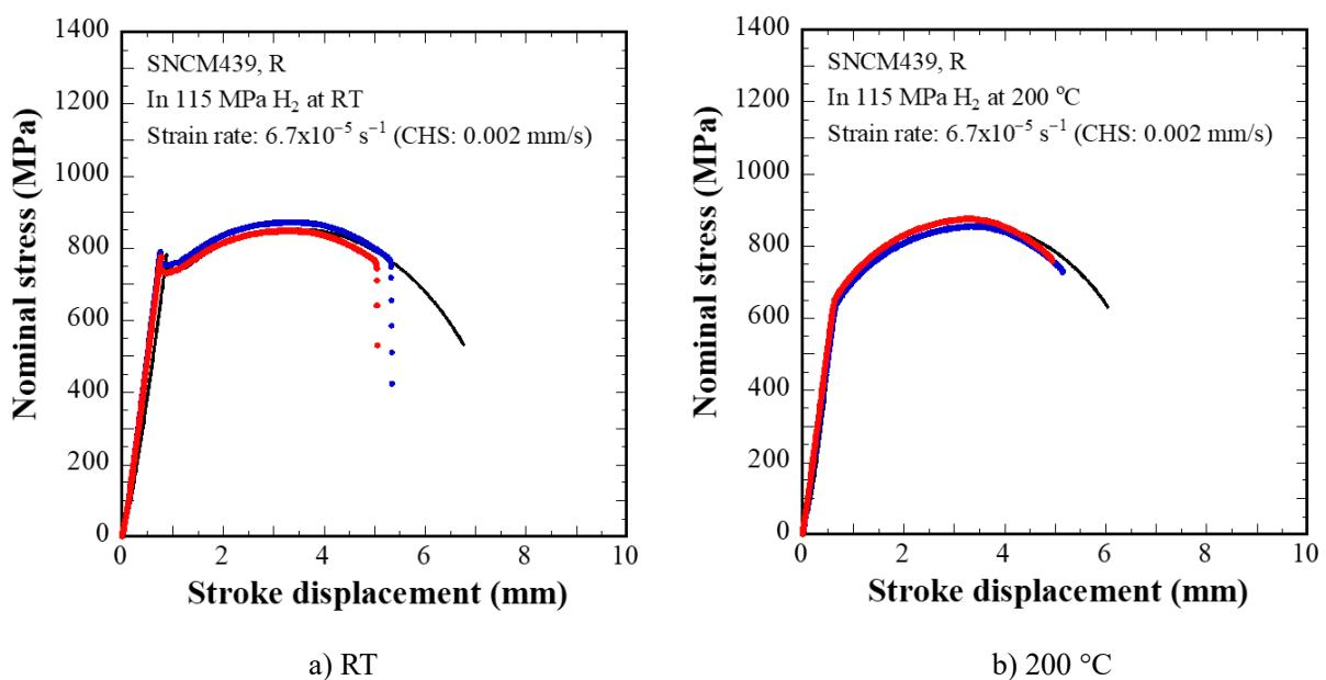
Fig. C.1.4.5 Stress - stroke curves of SNCM439 Heat R.
