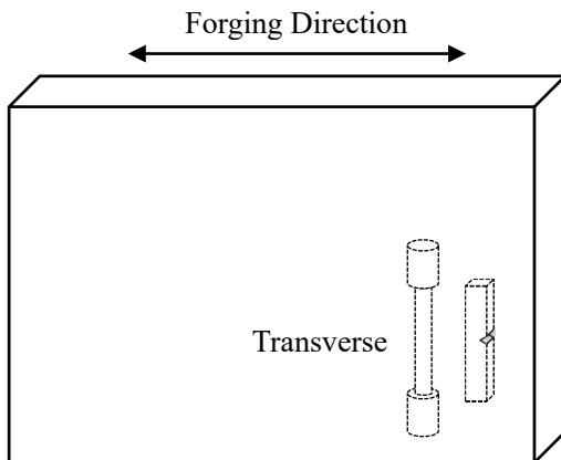
Fig. C.1.8.1 Schematic of specimen direction.
