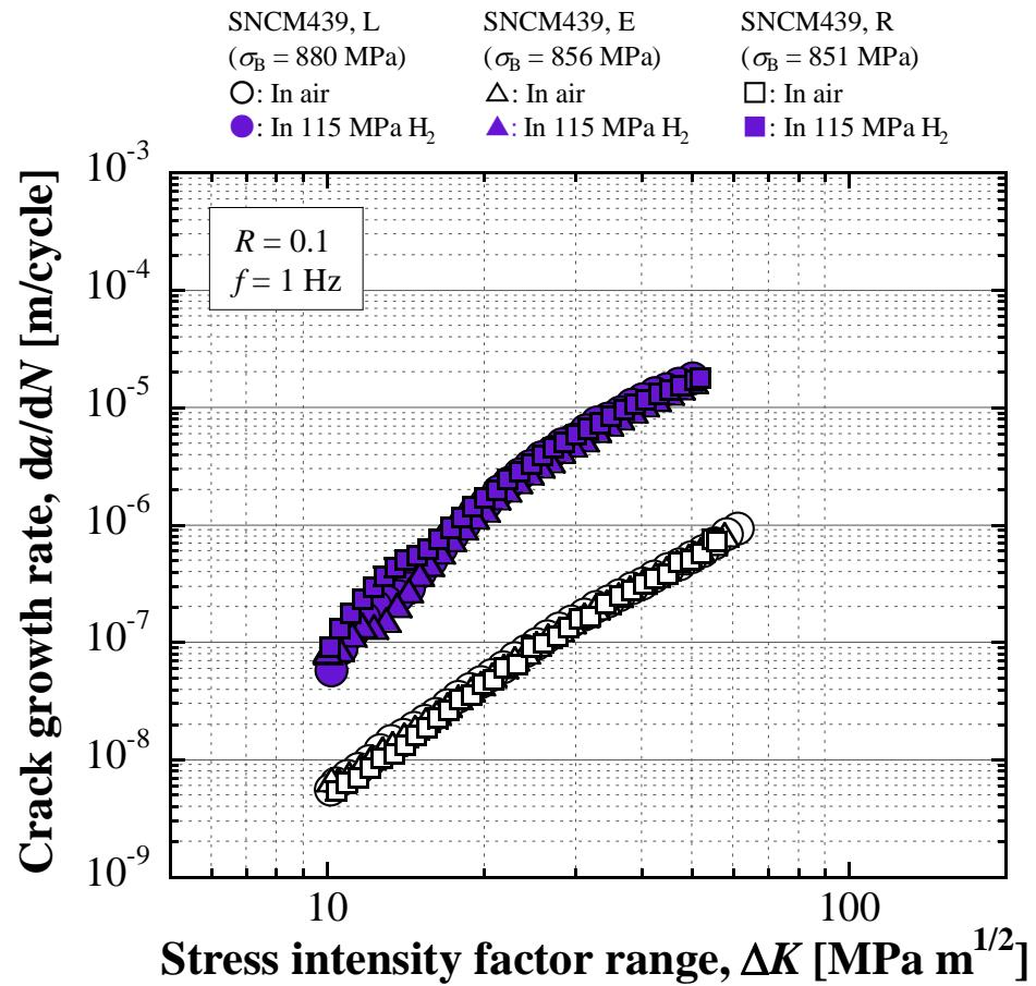
Fig. C.4.4.4 Relationships between  $da/dN$  and  $\Delta K$  for SNCM439.
