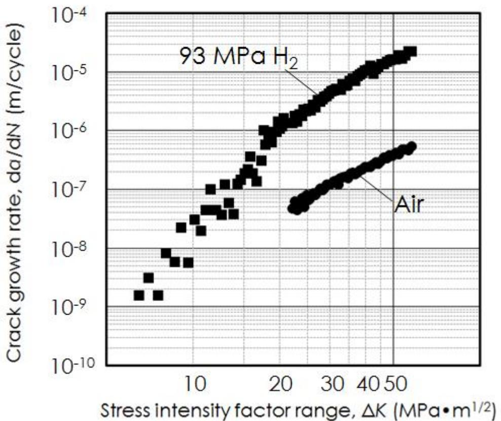
Fig. C.4.3.1 Relationships between  $da/dN$  and  $\Delta K$  of SNCM439.
