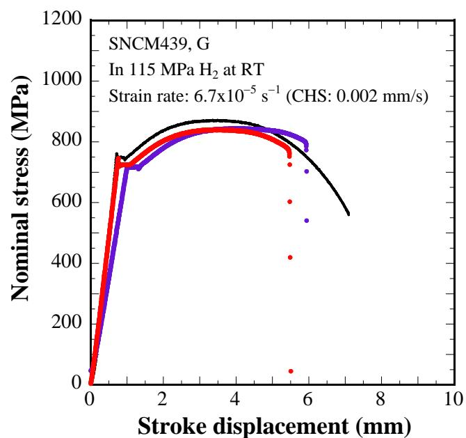
Fig. C.1.5.4 Stress - stroke curves of SNCM439.
