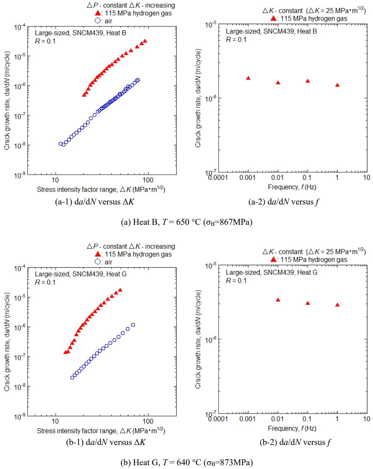
Fig. C.4.1.1 Relationships between  $da/dN$  and  $\Delta K$ , and between  $da/dN$  and  $f$  for large-sized SNCM439.
