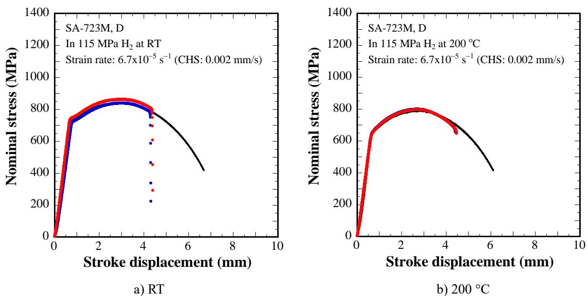
Fig. C.1.8.3 Stress - stroke curves of SA-723 Heat D.
