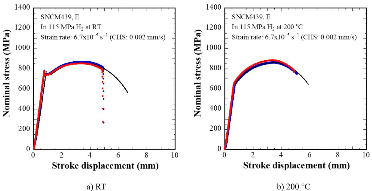
Fig. C.1.4.4 Stress - stroke curves of SNCM439 Heat E.
