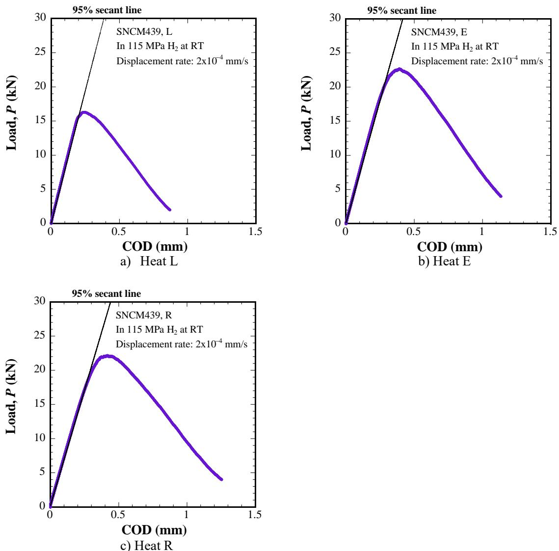
Fig. C.3.1.4 Relationships between Load and COD for SNCM439.
