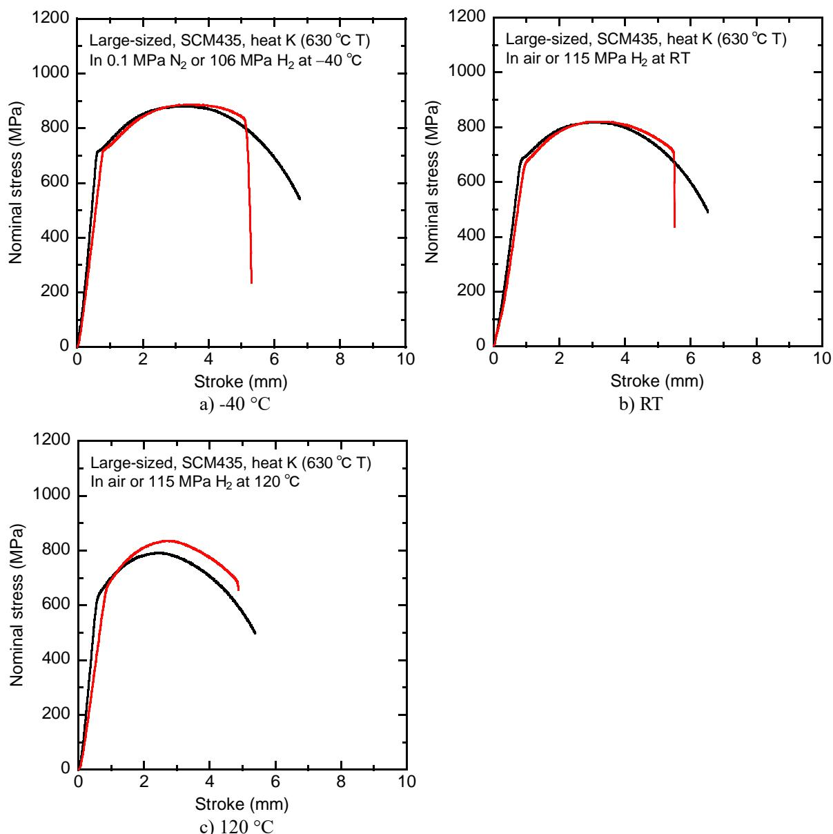
Fig. C.1.7.3 Stress - stroke curves of SCM435 Heat K.
