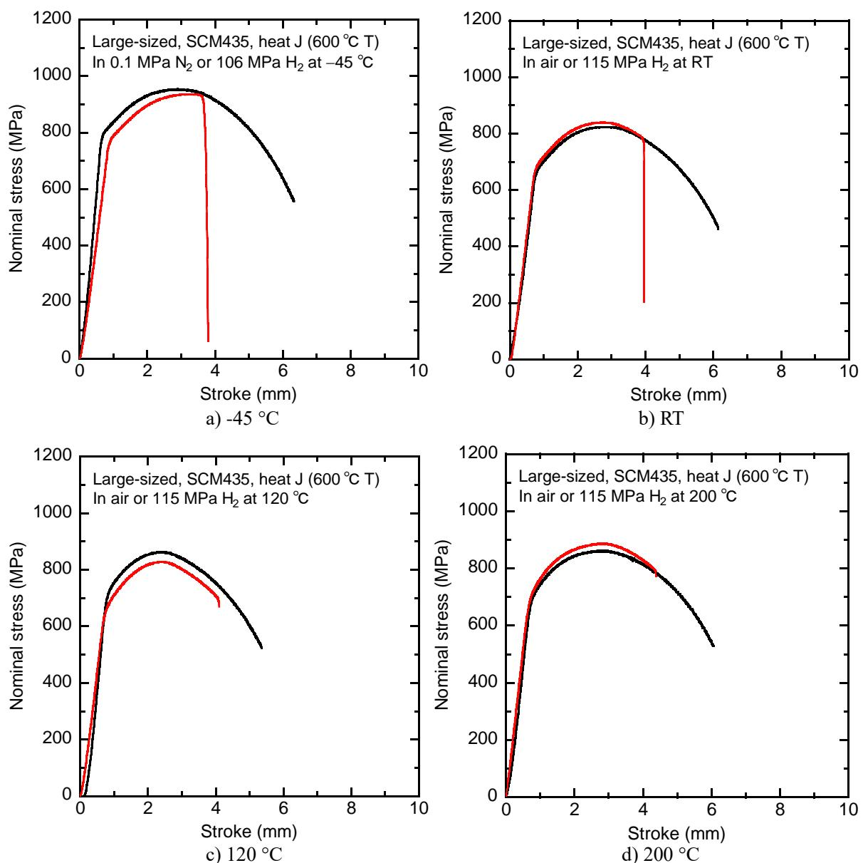
Fig. C.1.7.2 Stress - stroke curves of SCM435 Heat J.
