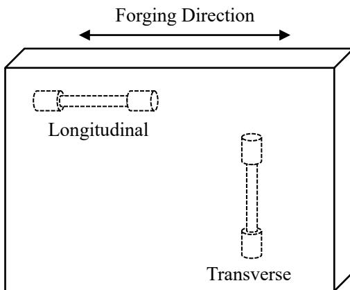
Fig. C.1.6.2 Schematic of specimen direction.
