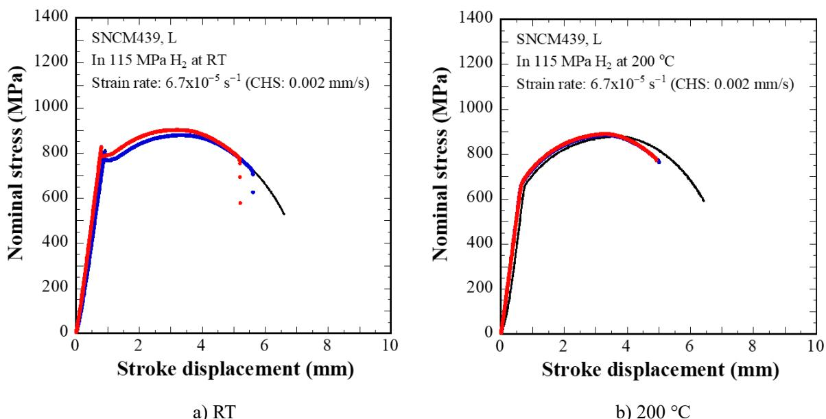
Fig. C.1.4.3 Stress - stroke curves of SNCM439 Heat L.
