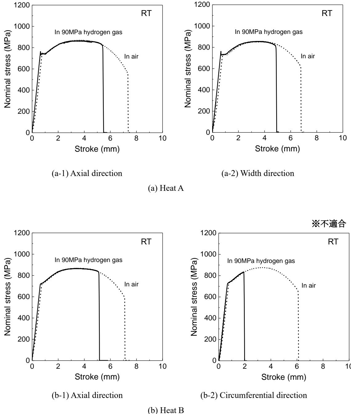
Fig. C.1.2.1 Stress - stroke curves of SNCM439.
