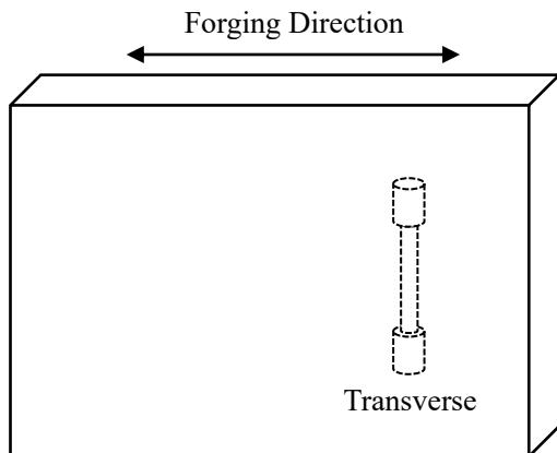
Fig. C.1.5.1 Schematic of specimen direction.
