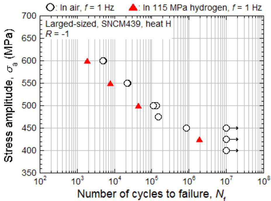
(b) Heat H, tempered at 640 °C ( $\sigma_B=873$  MPa)
