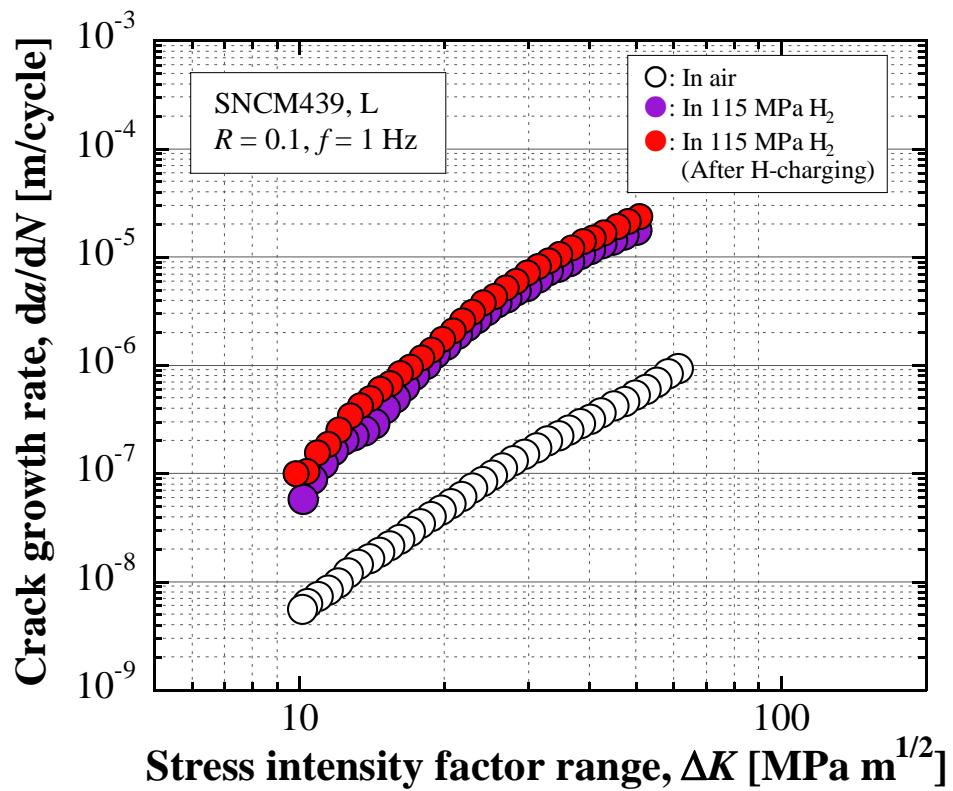
Fig. C.4.4.5 Relationships between  $da/dN$  and  $\Delta K$  for SNCM439 Heat L.
