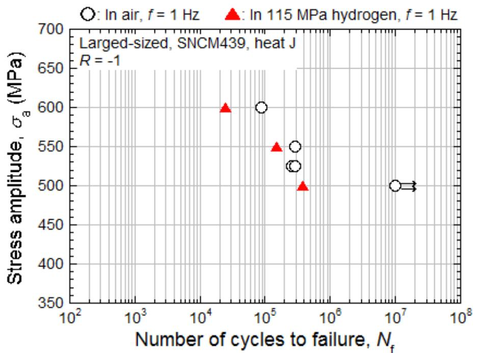
(c) Heat J, tempered at 620 °C ( $\sigma_B=1025$  MPa)
