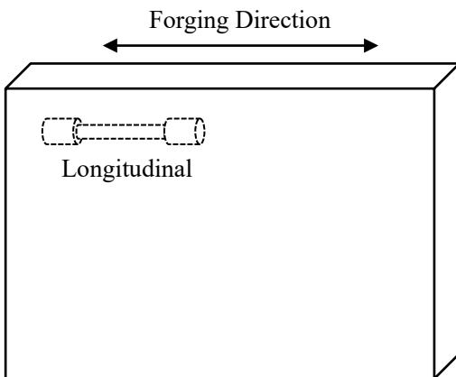
Fig. C.1.4.2 Schematic of specimen direction.
