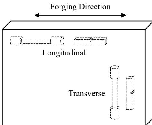
Fig. C.4.4.1 Schematic of specimen direction.
