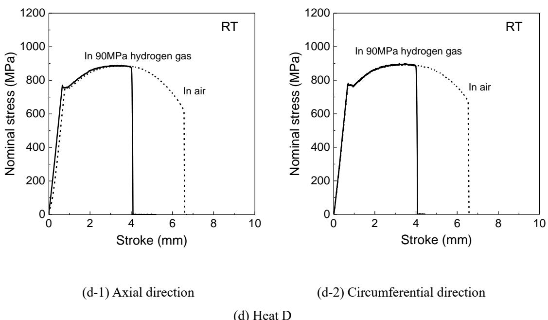
Fig. C.1.2.1 Stress - stroke curves of SNCM439.
