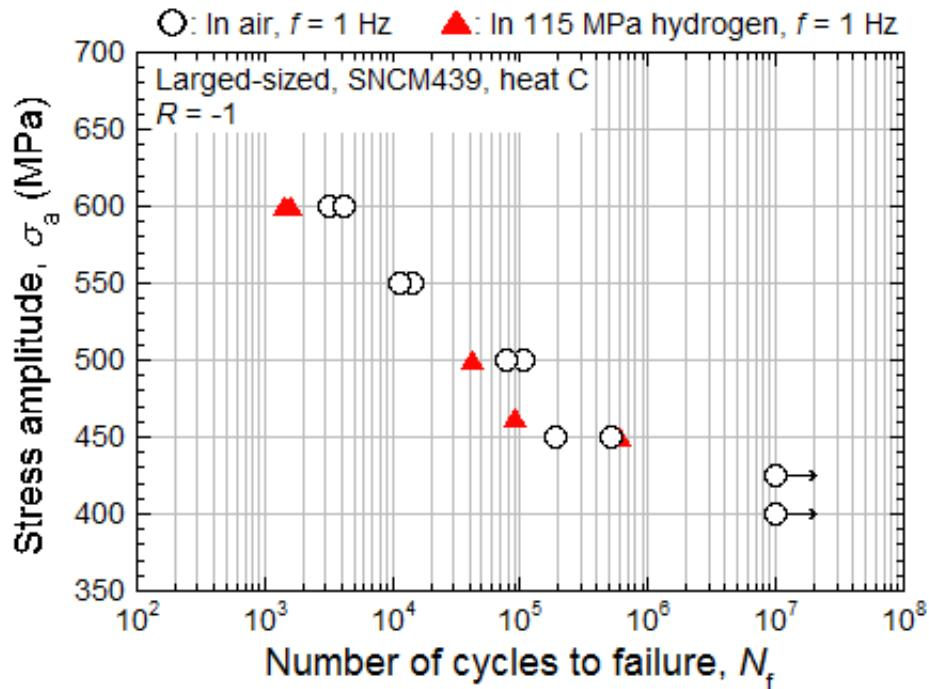
(a) Heat C, tempered at 650 °C ( $\sigma_B=867$  MPa)
