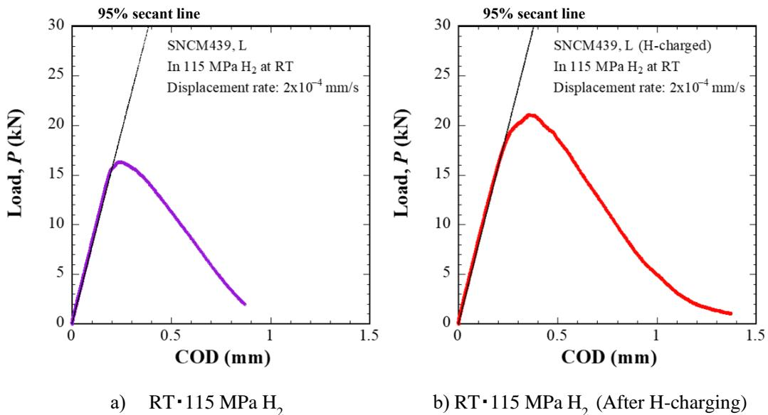
Fig. C.3.1.5 Relationships between Load and COD for SNCM439 Heat L.
