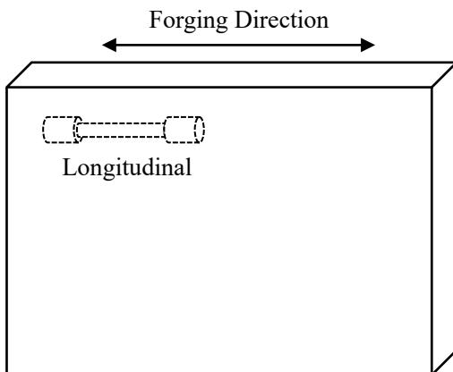
Fig. C.1.7.1 Schematic of specimen direction.
