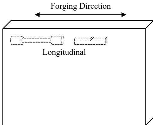
Fig. C.1.9.1 Schematic of specimen direction.
