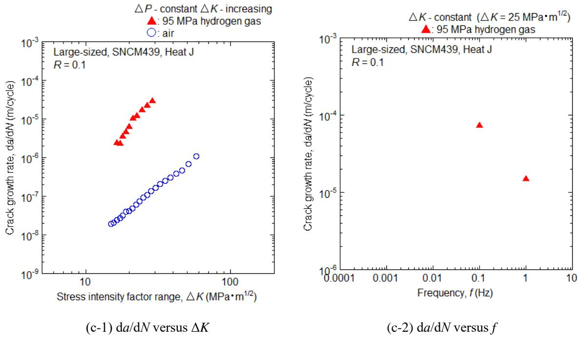
Fig. C.4.1.1 Relationships between  $da/dN$  and  $\Delta K$ , and between  $da/dN$  and  $f$  for large-sized SNCM439. (Continued)
