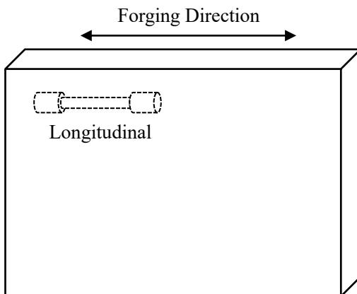
Fig. C.1.5.2 Schematic of specimen direction.
