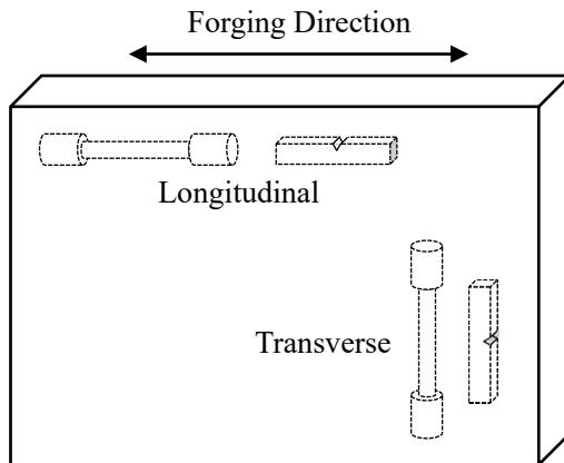
Fig. C.1.6.1 Schematic of specimen direction.
