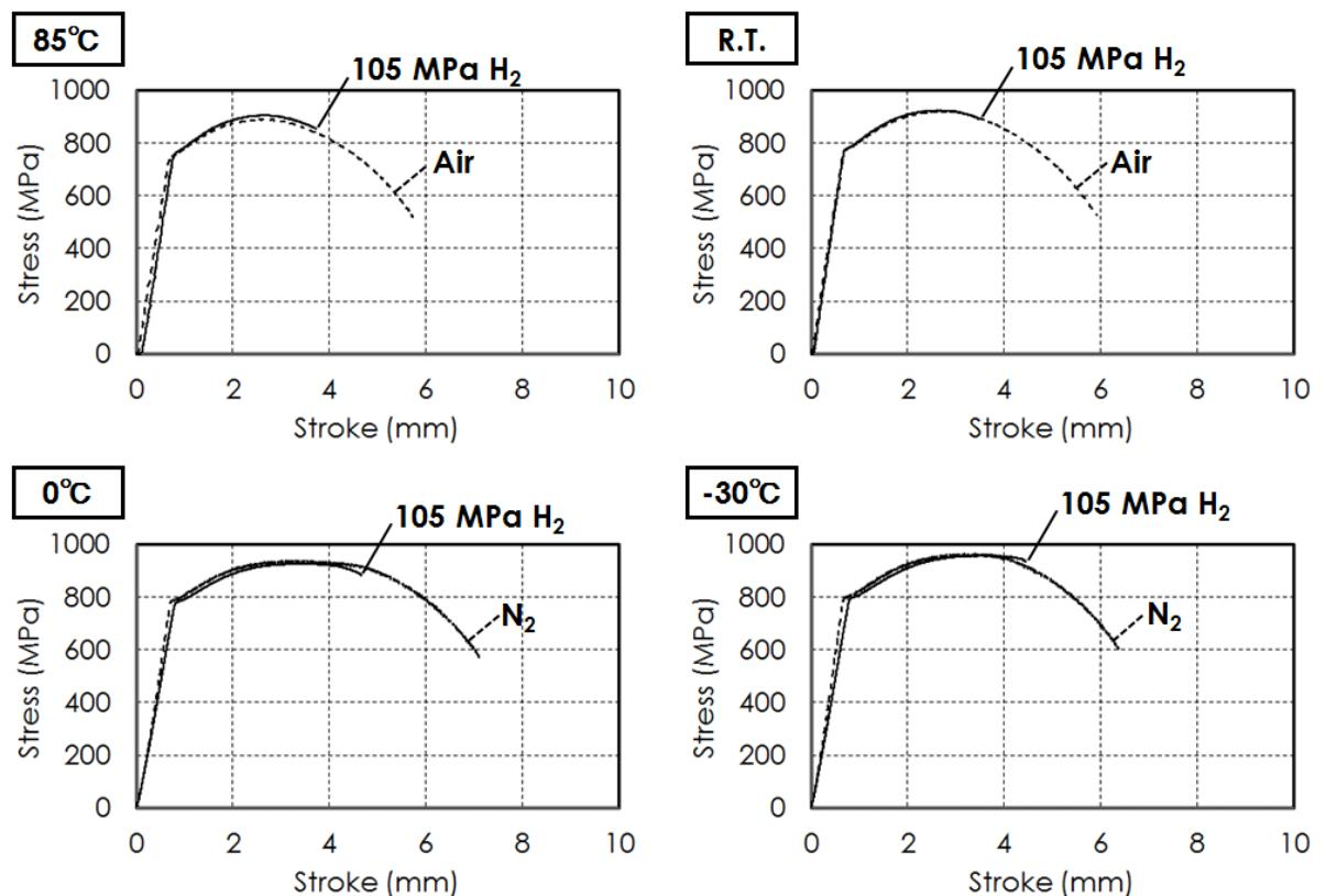
Fig. C.1.3.1 Stress - stroke curves of SNCM439.
