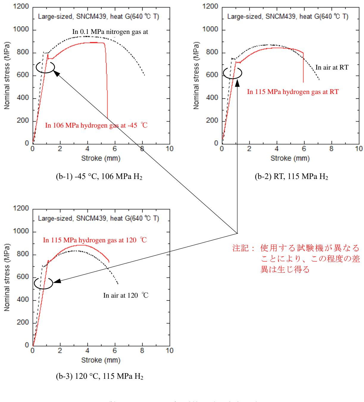
Fig. C.1.1.1 Stress - stroke curves of large-sized SNCM439 in 106 and 115 MPa hydrogen gas.
