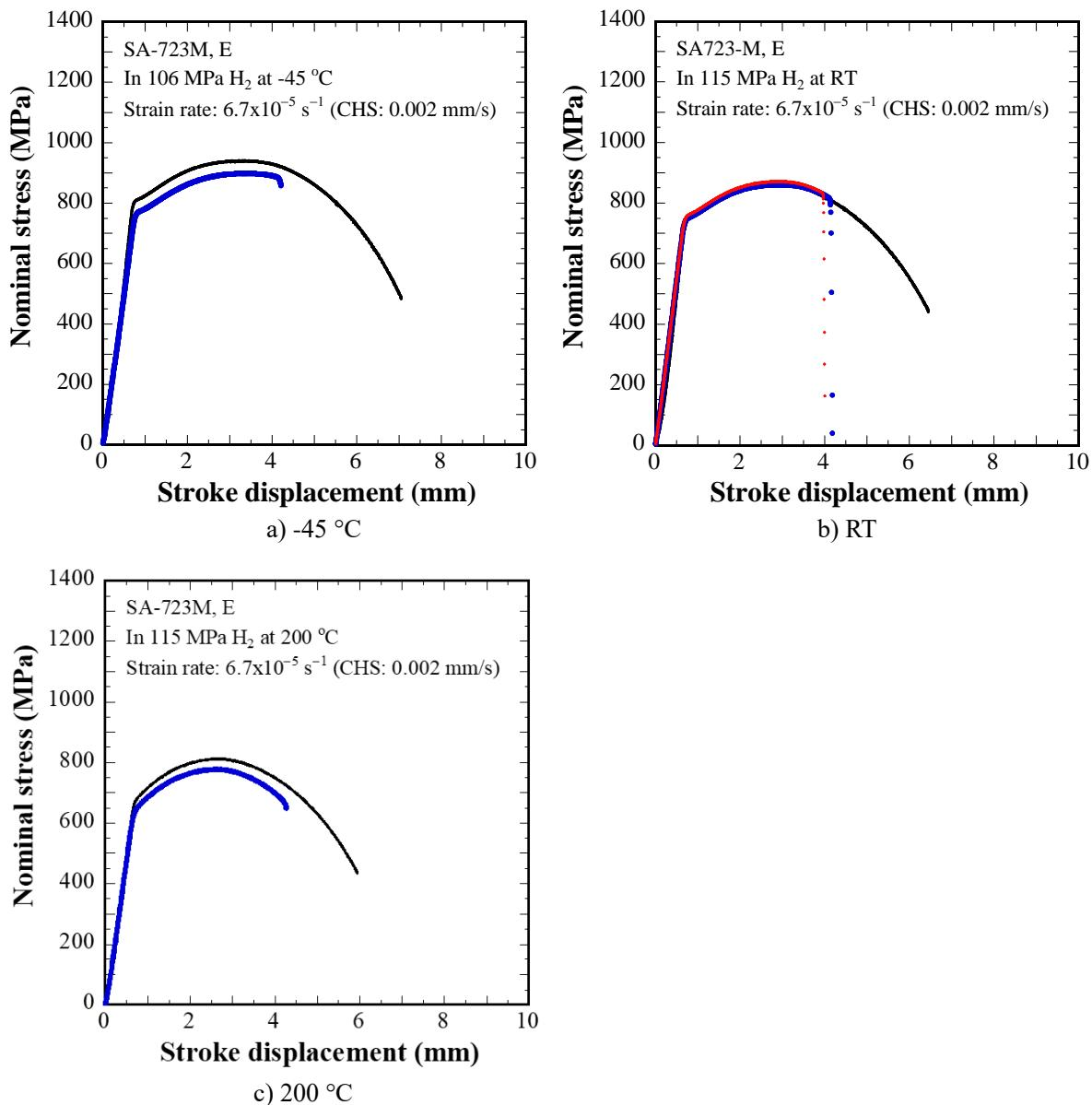
Fig. C.1.8.4 Stress - stroke curves of SA-723 Heat E.
