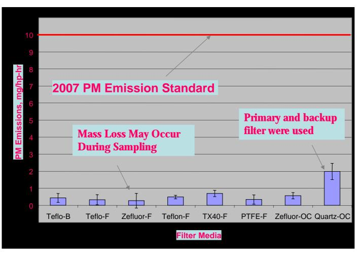
Filter Weight gain for the Teflo filter media during an FTP transient cycle was very low on the order of 5  $\mu$ g, with a coefficient of variation of more than 50 percent.
