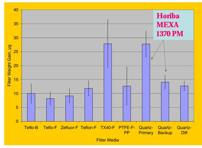
TX-40 Filter Media Collected 2.5 times higher PM than the Teflon Membrane Filter Media At this engine operating condition, the PM is likely dominated by sulfuric acid.
