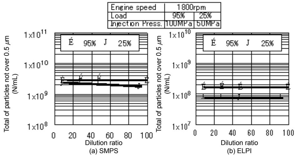
**Figure 2.1-4 Effect of dilution ratio on total particle count**
