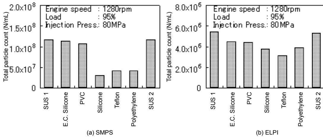
Figure 2.1-1 Effect of differences in sampling tube material on particle size distribution
