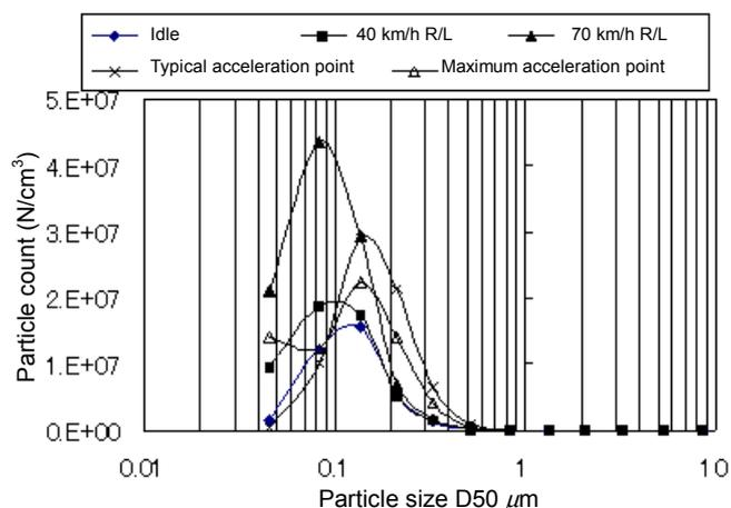
**Figure 2.3-3 Particle size distribution under each operating condition**
