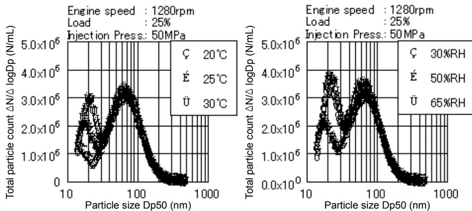
**Figure 2.1-3 Effect of diluted air temperature and humidity on particle size distribution (SMPS)**
