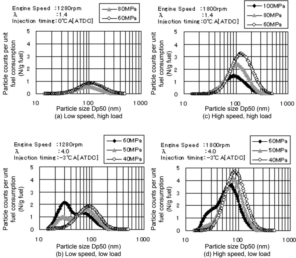
**Figure 2.2-1 Effect of fuel injection pressure on particle size distribution**
