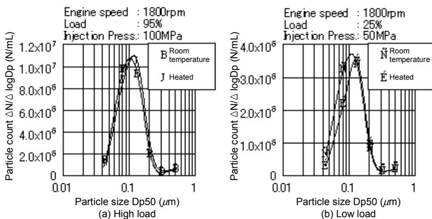
**Figure 2.1-6 Effect of ELPI unit temperature on particle size distribution**
