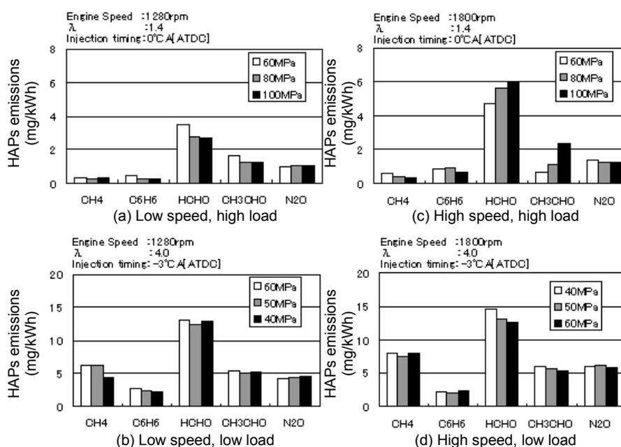
Figure 2.2-3 Effect of fuel injection pressure on HAPs emissions
