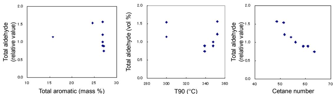
**Figure 2.3-1 Fuel properties versus aldehyde emissions**
