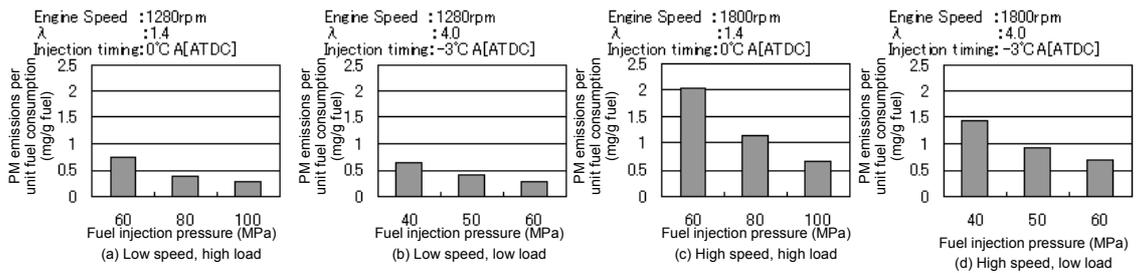
**Figure 2.2-2 PM emissions per unit fuel consumption**
