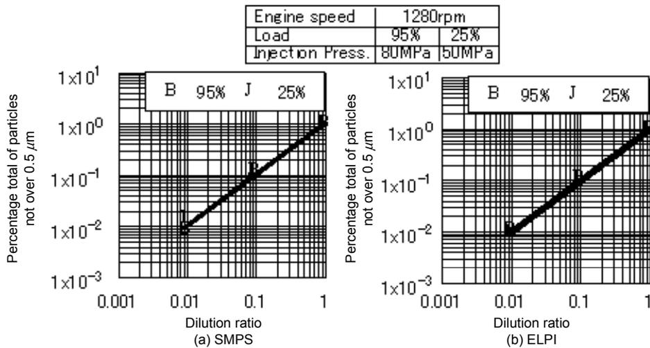
**Figure 2.1-5 Dilution ratio versus total particle count percentage**
