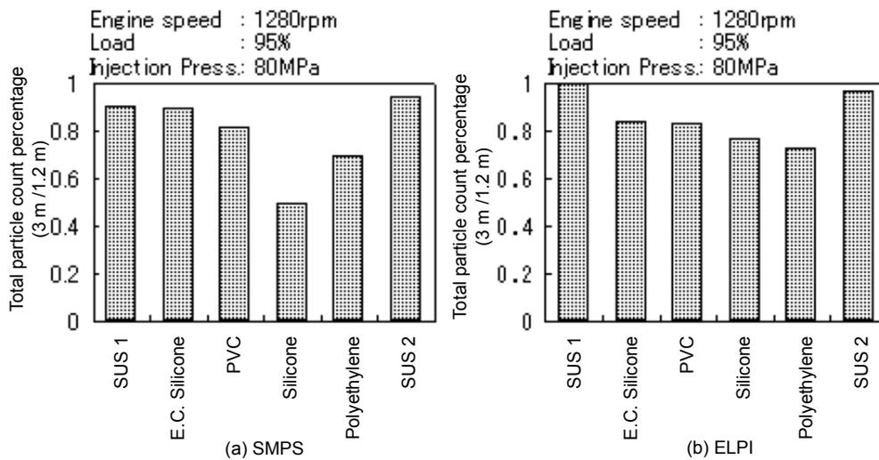
Figure 2.1-2 Effect of sampling tube length with each sampling tube material
